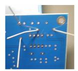
Solder one end and recheck that the resistor is seated on the board before soldering the second lead. If not, adjust before soldering.
