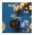
The outline of the package on the board should be used as a guide to orient the transistor.
