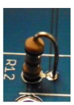
Solder one lead and recheck that the resistor is seated to the board.
