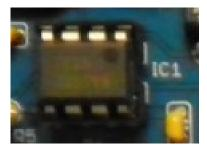
Note that you may need to form the leads on the ICs to align with the socket. If this is necessary, do so carefully to avoid breaking the IC leads.
