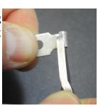
The ring terminal should fit into the u shaped area formed by opening up the crimp area on the ring terminal. Before crimping down, apply a small amount of heat sink compound to the diode body.
