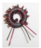
When winding, each time the wire passes through the toroid center counts as a turn. For example, just passing a wire from one side to the other of the toroid counts as a turn even though, it does not wrap around the toroid. When completed, it should look like the photo on the right.
