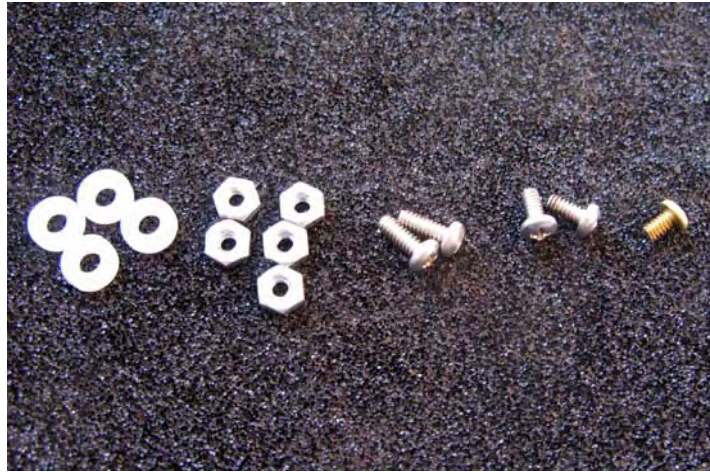
From left to right: Nylon washers, 4-40 nuts, 5/16"L screws, 1/4"L screws, 3/16"L Brass screw
