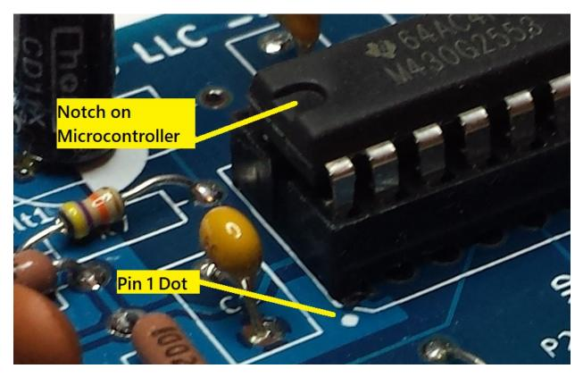
Above is a picture of the Pin 1 end of a microcontroller.
