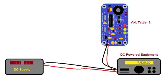
Setting up VoltTattler 2 at the equipment can alert an operator to voltage drops between the power source and your equipment. In addition hearing the "roger" beep (Morse 'R', .-.) can audibly alert you if the power dropped out completely and then came back again (intermittent connection). This can be very useful in troubleshooting a system.
