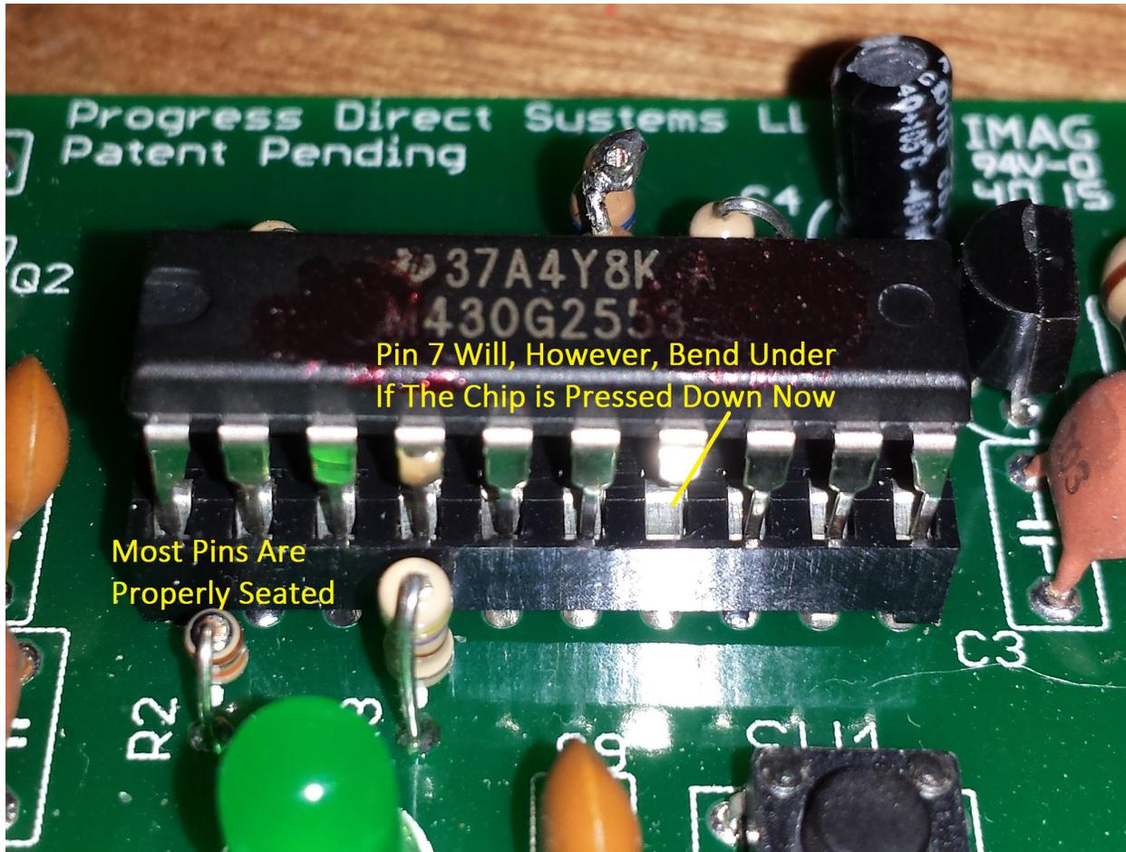
Here the builder is headed for trouble. Pin 7 of the chip is not pointing down into the socket but tucked a bit back under the chip. When they push down on the chip to seat it into the socket, pin-7 will fold under the chip and not connect. This may cause issues even though the chip seemed to seat solidly. Check each pin for proper direction before attempting to seat the chip into the socket.
