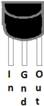
If there is 5 volts or more at the **In** pin of the LP2950 check that the **Gnd** pin is at 0V and that the **Out** pin is at about 3.3V. If the **Out** voltage is 0 or below 3V there may be a short on the output. Look for traces that have shorted. If it is high (> 3.5V) be sure that the **Gnd** terminal is near 0V.
