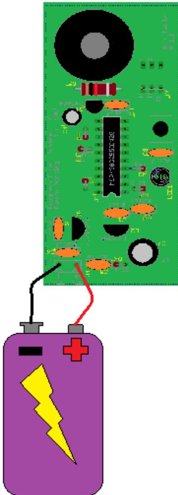
First connect the new Volt Tattler to one of the 9-volt batteries. As always watch polarity. If the battery is relatively alive the Volt Tattler should sound the Morse 'R' (-.-) then repeated Morse 'L' (-.-.). In addition the heartbeat LED should flash periodically.
