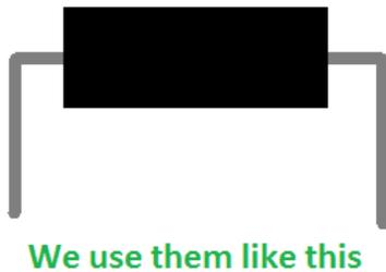
When we get the chips the leads are usually splayed out on an angle. This promotes proper tension for automated insertion machines but causes grief trying to manually install the chips into a board or socket. Use your work surface to bend all of the pins at the same time while keeping them in line.
