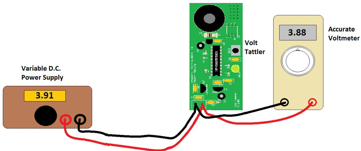
1. Connect the variable power supply and the voltmeter to the VoltTattler in parallel as in the accompanying diagram. VoltTattler will begin blinking the heartbeat LED and send a Morse "R" (-.). That "R" may be followed by continuous "H"s (.... .... ....) or "L"s (-.. -.. -..) depending on the supply voltage and limits currently set in the VoltTattler unit. This is no matter as we plan to calibrate the unit.
