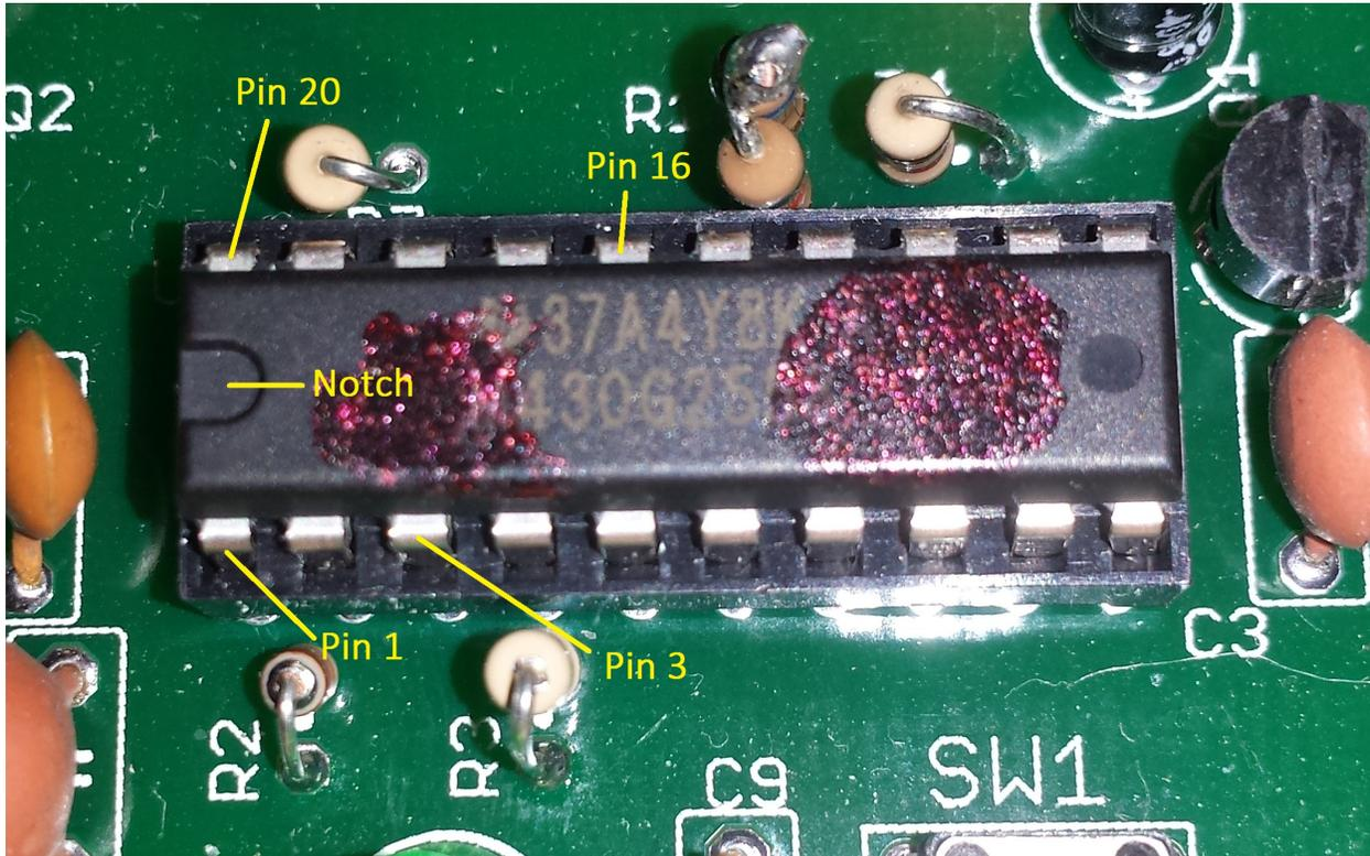
Carefully aligning the pins can prevent bending a pin off to the side or underneath the chip. Be sure that all of the pins are through the board and ready to be soldered to the pads on the back of the board (the non-component side). Once all pins are seen through the PC board, use a piece of cellophane tape to temporarily secure the chip for soldering.
