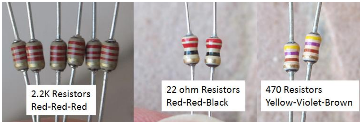
Figure 15. Perform visual inspection to make sure all resistors are the same value
