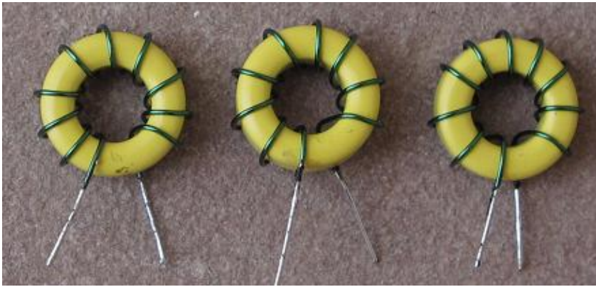
Figure 35. Example of 15m coil set L3 (10T), L4 (9T), L5 (10T)
