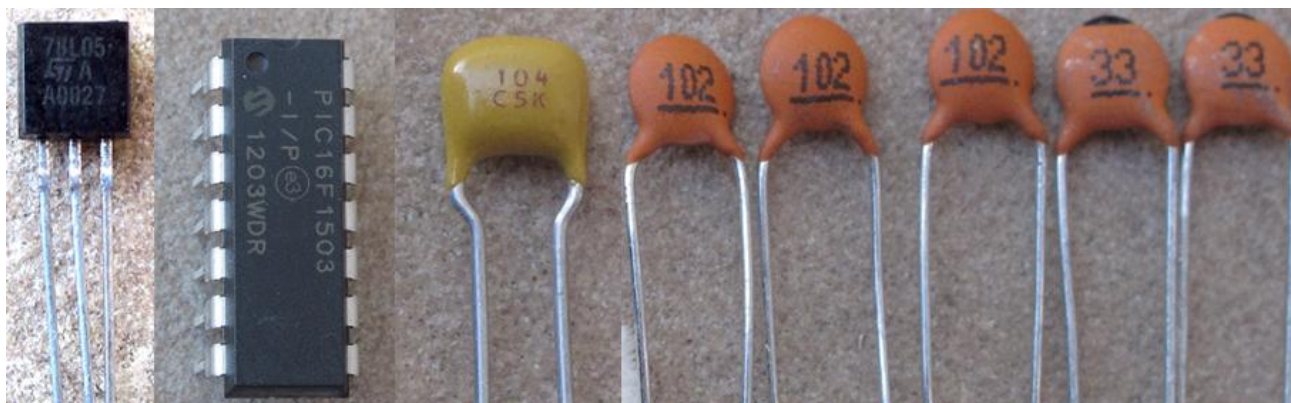
Figure 23. Picture of parts: 78L05 and PIC16F1503 plus 0.1 uf (104), 1000 pf (102), and 33 pf caps
