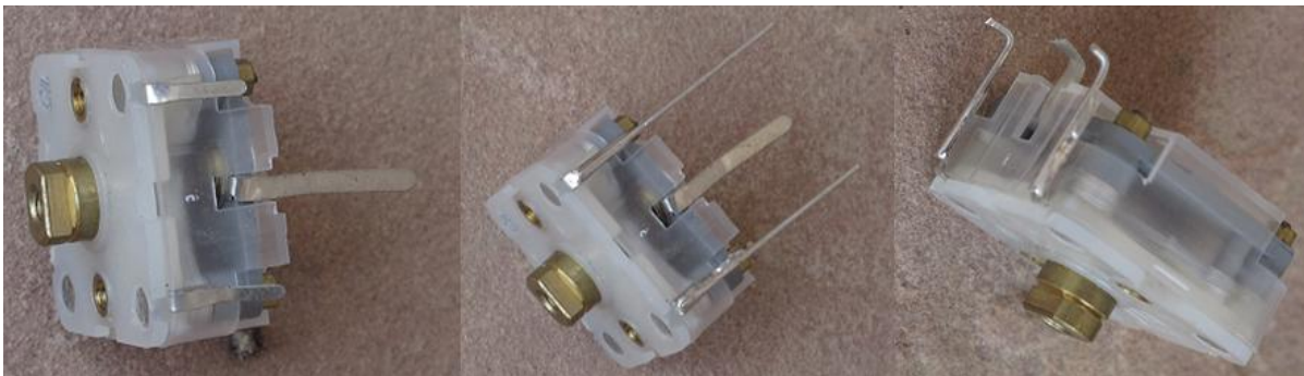
Figure 40. Polyvaricon with short leads. Leads extended with resistor leads. Form and clip leads.
