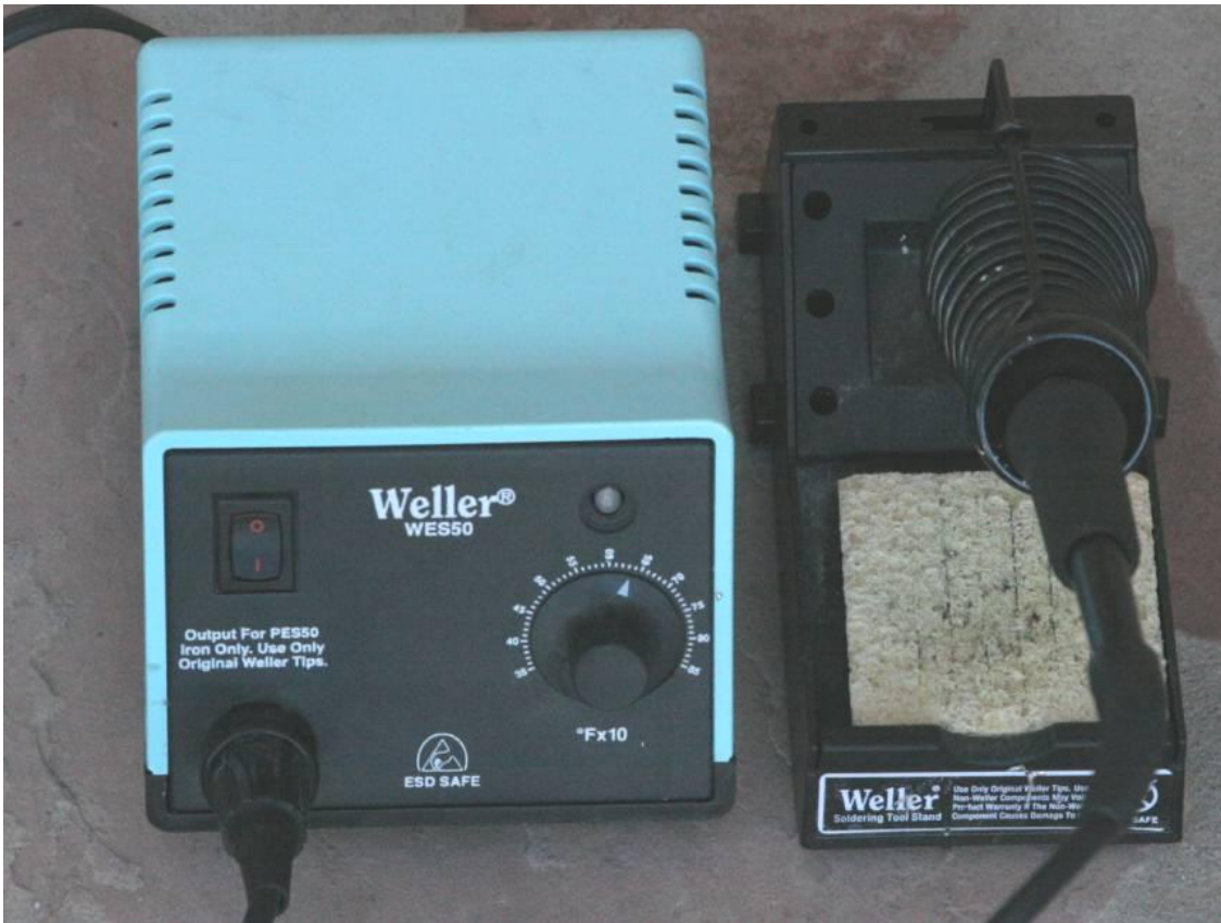
Figure 2. A temperature controlled soldering helps a lot. 750 degrees is recommended for non-lead tinned boards
