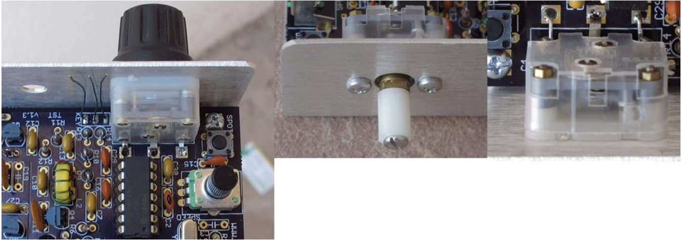
Figure 41 Mounting of C1. Mount C1 on the front panel first, then solder the leads from the top side.
