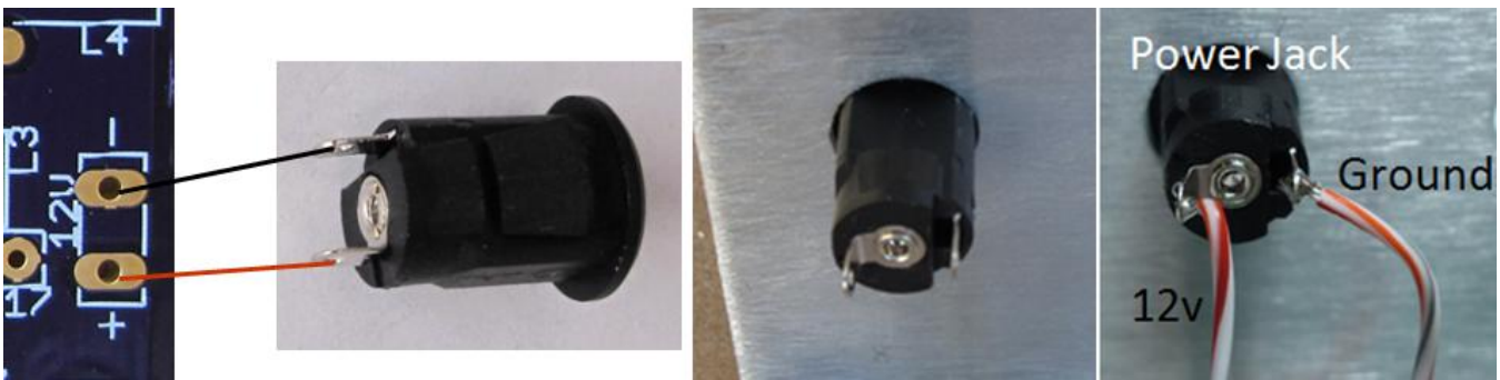
Figure 42. Visualization of rear panel 12v power jack. Power and ground connections shown. Hookup wire used.
