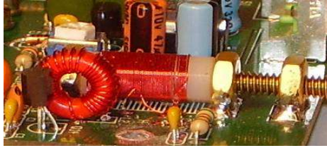
Finished PTO coil mounted to board.
