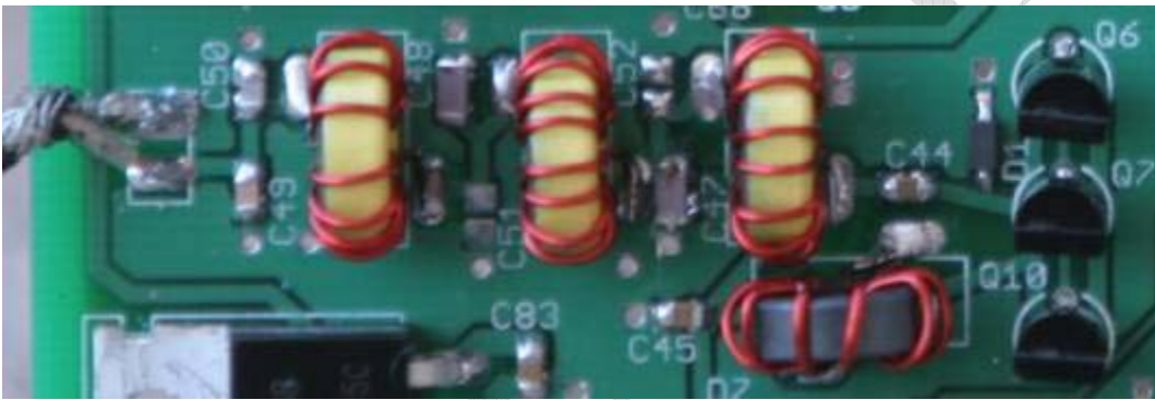
Figure 60. Top side parts view of the PA circuit. C50 (left top end cap) not used on the 30m version.
