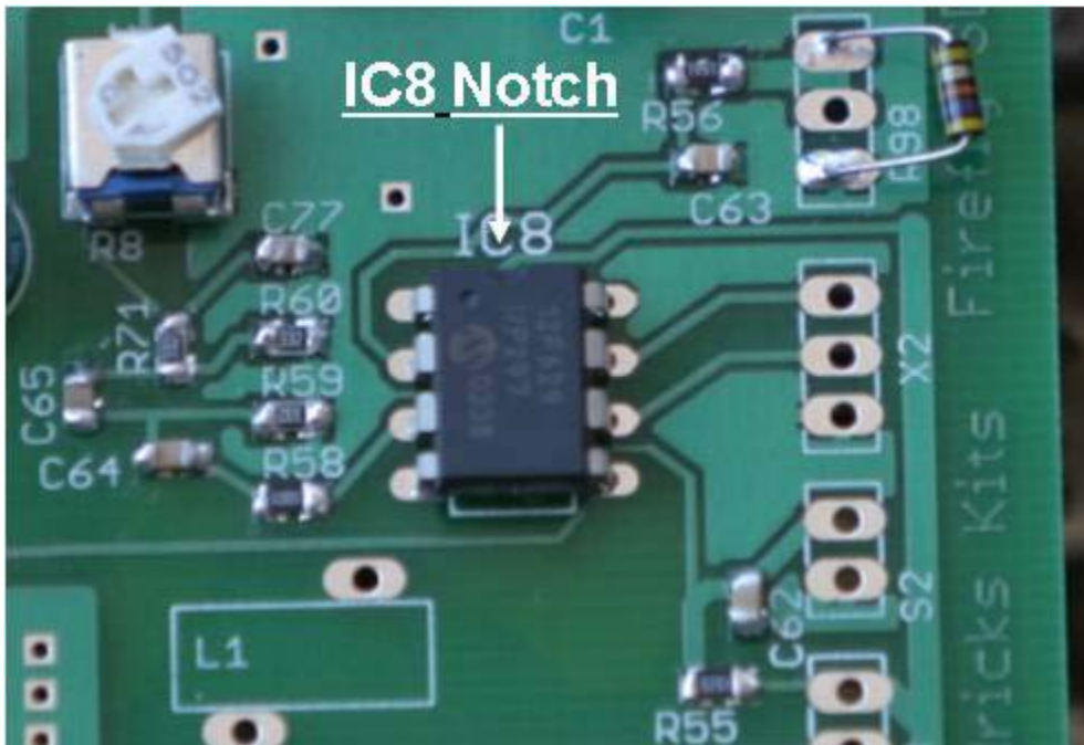
Figure 26. Top side keyer parts. Note the orientation of IC8. IC8 Notch is at the top end.
