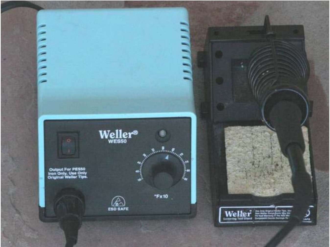
Figure 2. A temperature controlled soldering helps a lot. 750 degrees is recommended form non-lead tinned boards
