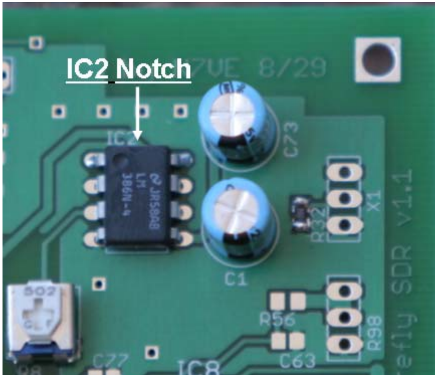
Figure 22. Top side IC2, C73, C1, volume trim pot R8 and R32. Note IC2 polarity and black stripes on C1 and C73.
