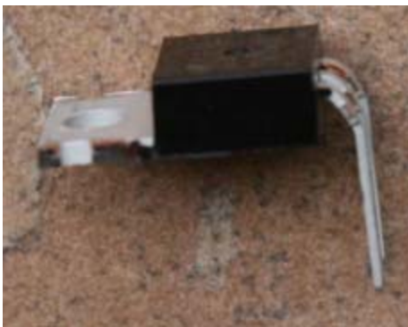
Figure 16. Lead forming of the LM78M05 5v regulator before installation
