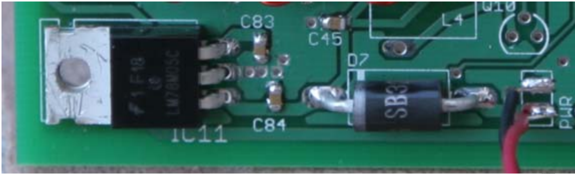
Figure 15. Top side view of 5v regulator, protection diode, and 9v temporary connection. Note D7 diode polarization!
