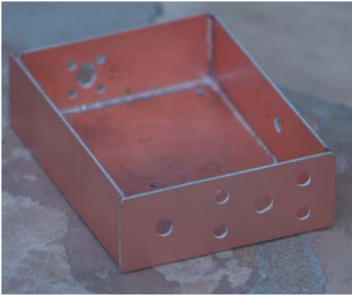
Figure 75. Homebrew case fashioned out of double sided PC board, 5" x 3.5" x 1.375".
