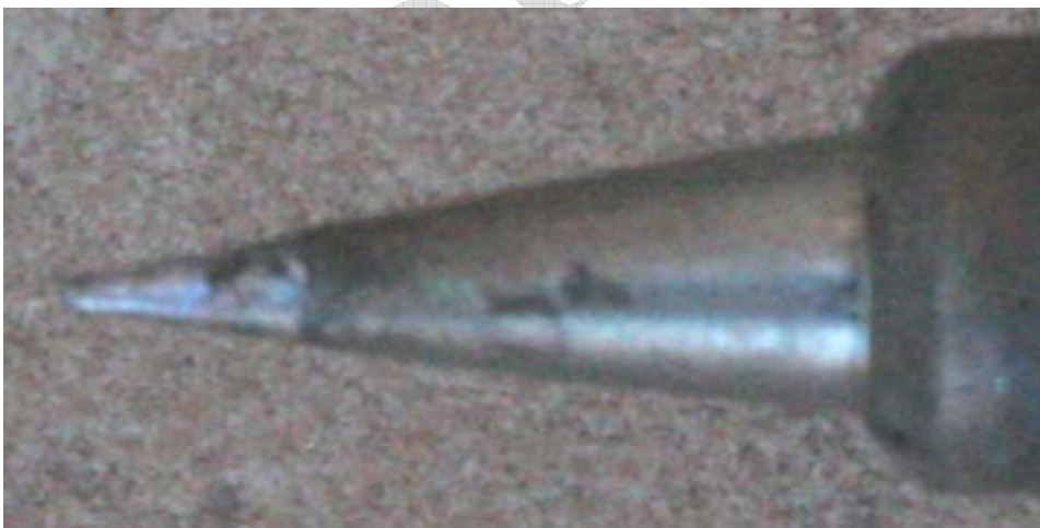
Figure 3. A very pointed soldering iron tip is a very big help for small surface mounted components
