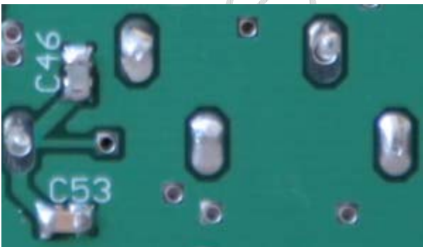
Figure 61. Bottom side part view of PA circuit. C53 not used in the 30m version
