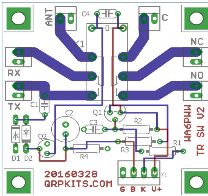
Note: Pin 1 of X1 is the pad closest to the X1 Label (on the right above) and is the connection point for 12V power. The leftmost pin (4) is ground connection.
