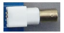
After the first support pin is soldered, recheck that the connector is seated on the board. If not, reheat the connector support pin while pressing down on the board to fully seat it.
